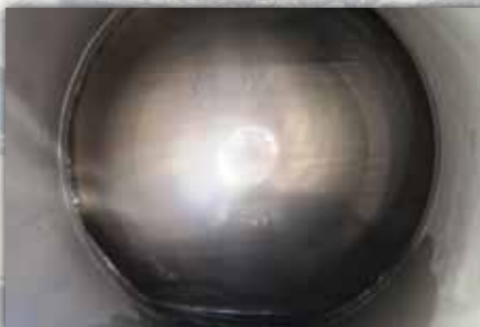
Close-up view of primary sealing surface of closed ball after approximately 1500 cycles at 2700 psig differential pressure
